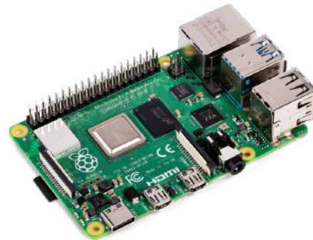
Figura 15 - Raspberry Pi 4B, 8GB
